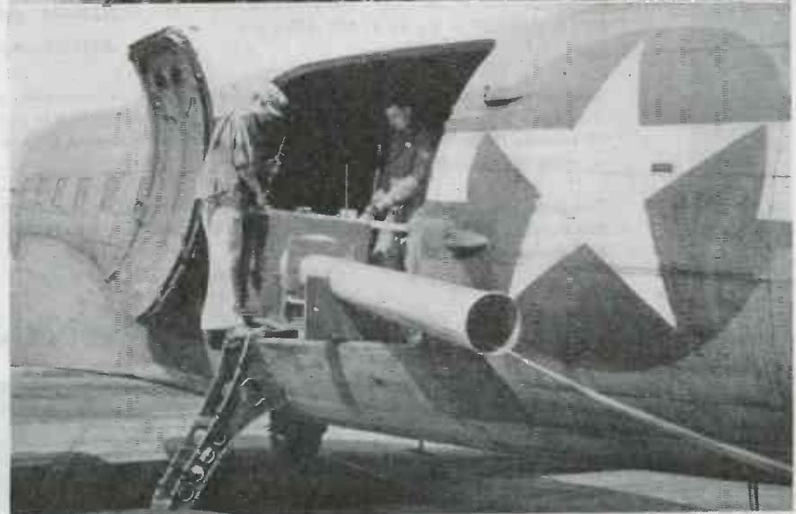
Looking inside the airplane at the series of special containers for the reels of wire that are fed out through the pipe illustrated in the lower view
