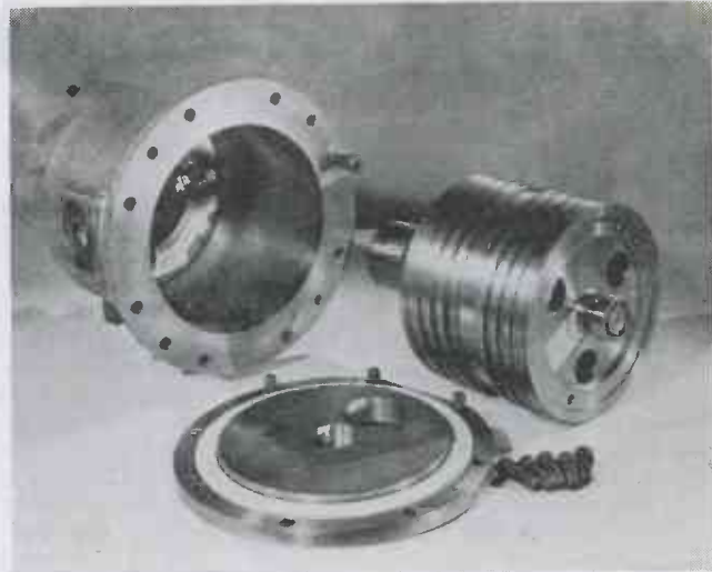
Fig. 6—Molecular pump, backed by Megavac pump, exhausts oscillograph chamber in from 7 to 10 minutes to a lower pressure than necessary. Vacuum pressure is then adjusted by valving in a small amount of air
