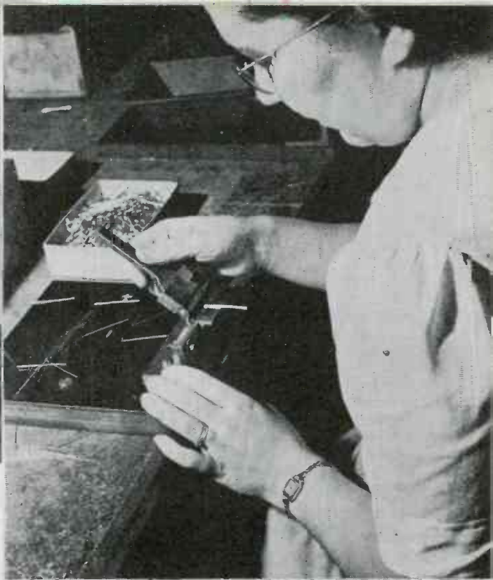
Heading many in-line rivets is eased by a slide with multiple anvils at the Westinghouse Sunbury plant. Spring loaded balls rise into counterbores for right location
