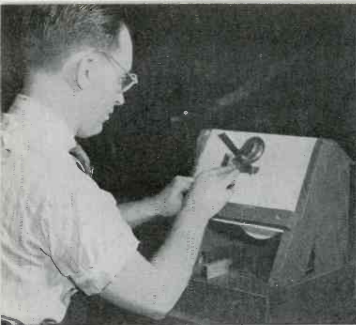
Illuminated ground glass inspection surface developed at General Electric plant for checking angles on tools and cutters is much better than holding work up to the light
