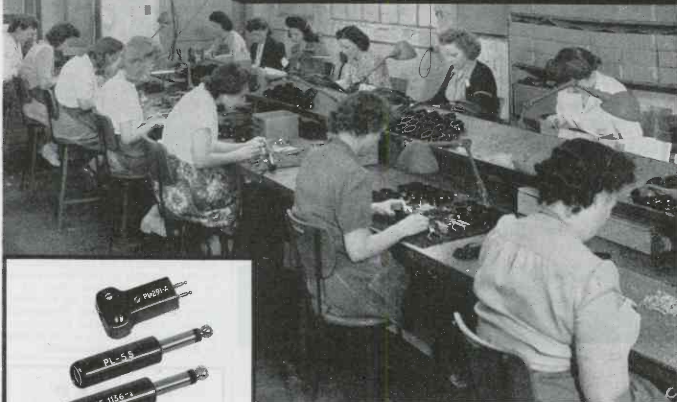
Marine microphone assembly. Plastic and metal parts designed, made and assembled by Remler to meet Navy and Merchant Marine specifications.
